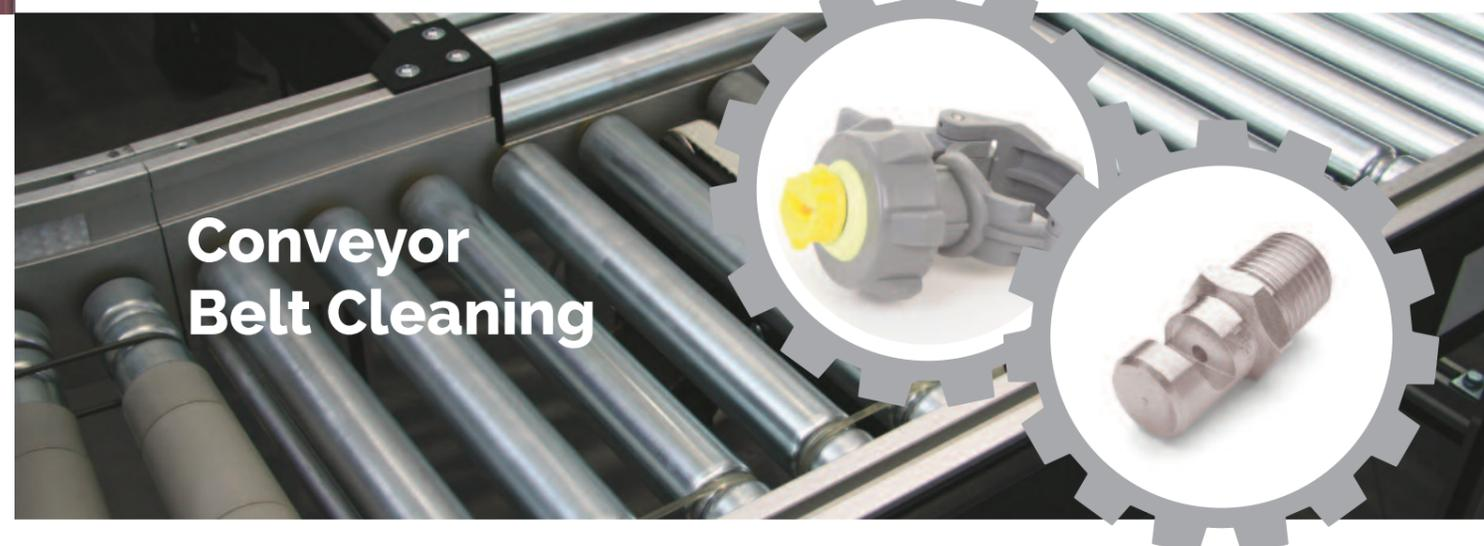
Conveyor belts carrying food products require regular cleaning to ensure that hygiene standards are maintained. Cleaning efficiency can be improved significantly by using fixed spray nozzles in place of manual operator based cleaning.
